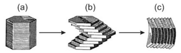
Figure 1. (a) Hexagonal ice crystal with glide planes parallel to the base. In lake ice the c-axes of the crystals are vertical and the glide planes parallel to the water surface. (b) Crystal deformed plastically by shear stress parallel to the glide planes. (c) Elastic deformation of crystal by strain normal to the glide planes.
